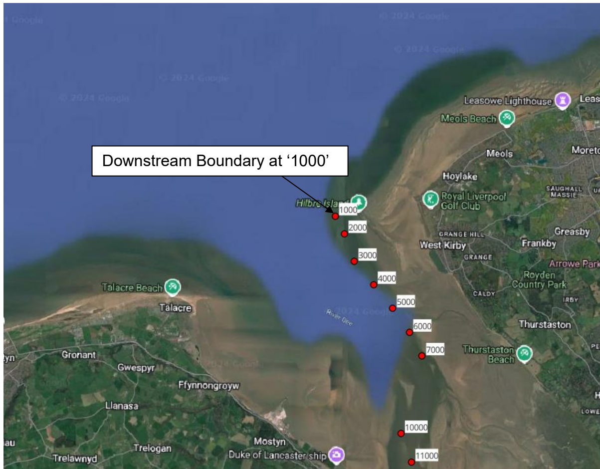
Figure 3: Model downstream boundary located at the Mouth of the Dee ("1000" has been used for the boundary location) (Source: Google Earth, accessed October 2024)
